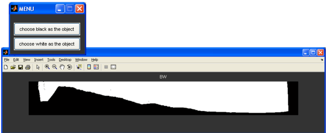
Figure 2. The first part of the GUI is composed of two windows. The current image is presented after its conversion to black & white (BW) image (bottom window). The upper window is a menu in which the user chooses if the object (the piece) is white or black.
