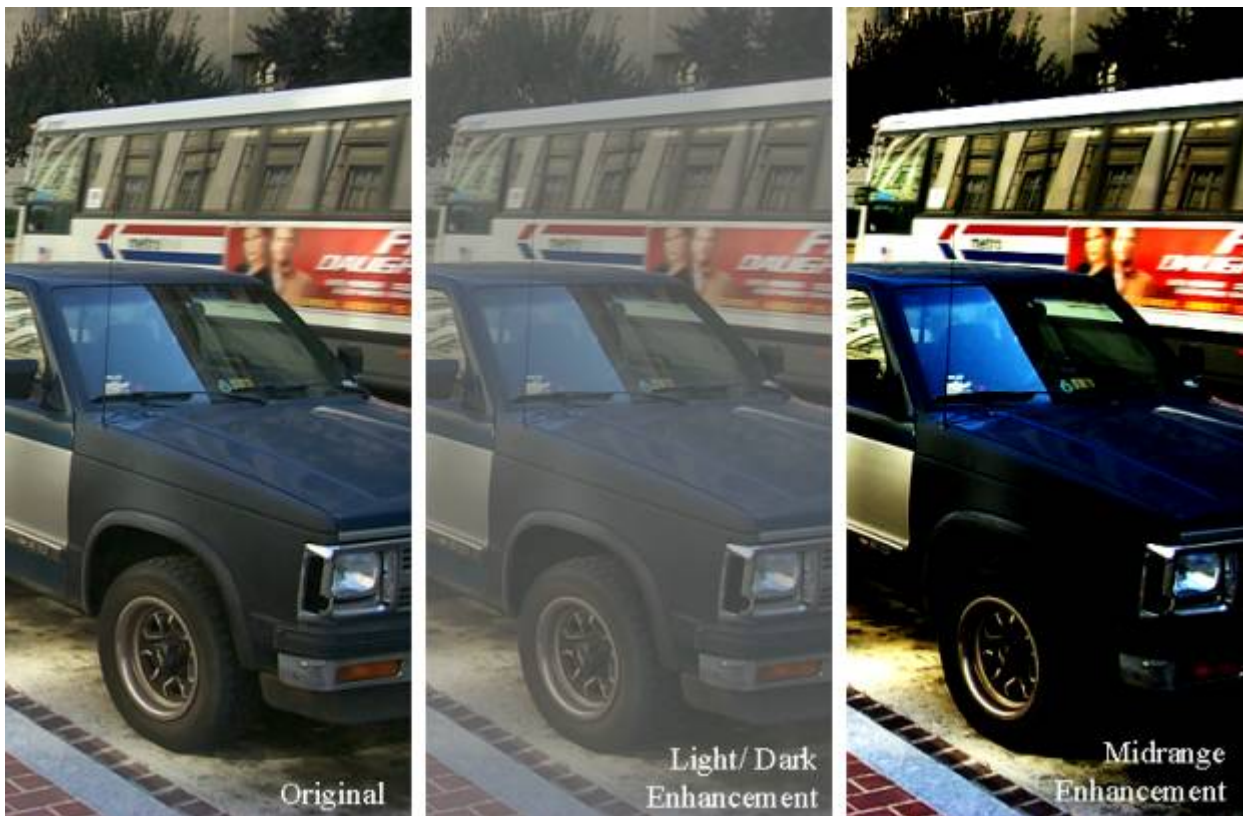
Figure 2. This example shows nonlinear contrast adjustments. Left: original image; Middle: enhancement of shadow and highlight areas, at the expense of midrange tones; Right: enhancement of midrange tones, at the expense of shadow and highlight areas.
