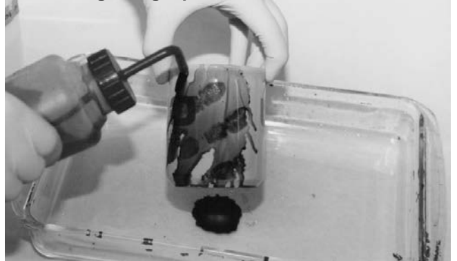
Chemical processing of latent fingerprints on a coffee mug using a protein stain.
