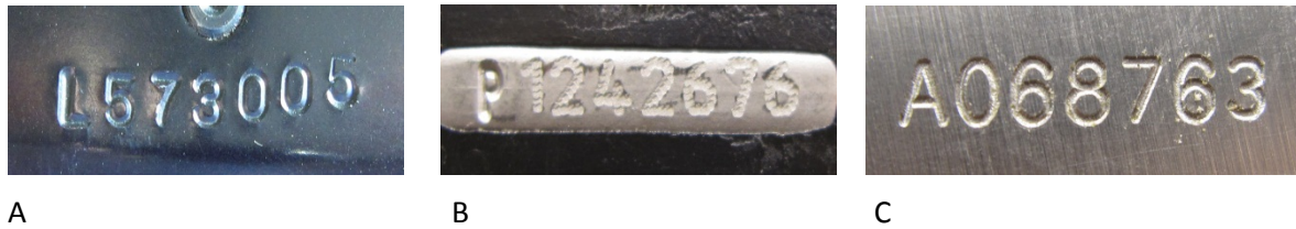
Figure 5. Stamping (A), Dot Peening (B), and Laser Etching (C) applied serial numbers showing differences in quality marks.
